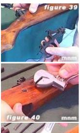
**40)** If you do not have an SVT tool you can if you are careful to not damage the **stock** use a pair of adjustable pliers to loosen and remove the **cross pin screw**.
