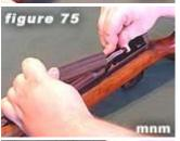
**75)** Compress **recoil springs** by pressing on **rear spring guide**. Place **rear spring guide** into slot inside rear of **receiver cover**.
