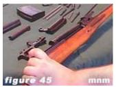
**45)** Return **receiver** and **barrel assembly** to **stock**.
