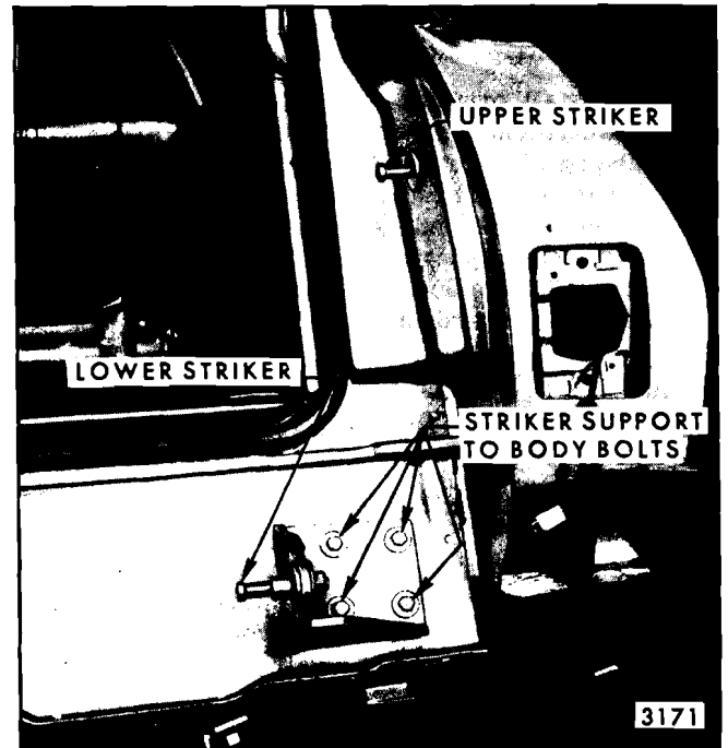
Fig. 9-31—Tail Gate Adjustments - "B" Body Shown "A" Body Typical
